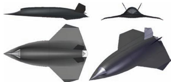
Fig. 3 Aerodynamic configuration of HSUAV
